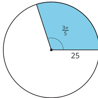
Additionally, we can write a formula for arc length based on the definition of radian measure:  $\theta = \frac{\ell}{r}$ , where  $\theta$  is the central angle measure in radians,  $\ell$  is the arc length, and  $r$  is the radius. Rewrite the definition to solve for arc length. We get  $\ell = r\theta$ .
