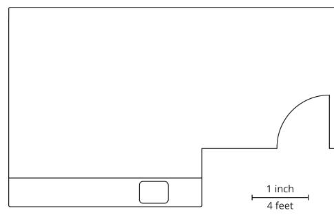
Suppose the longest wall is 15 feet long. We should draw a line 3.75 inches long to represent this wall, because  $15 \div 4 = 3.75$ .
