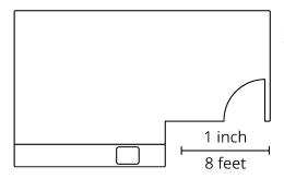
Notice this drawing is smaller than the previous one. Since one inch on this drawing represents twice as much actual distance, each side length only needs to be half as long as it was in the first scale drawing.
