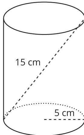
The volume of the cylinder is the area of the base multiplied by the height. This is  $25\pi \cdot \sqrt{125}$  cubic centimeters, or approximately 878.1 cubic centimeters.
