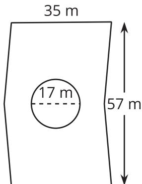
Each floor is the same chevron shape that is approximately 2 parallelograms put together, with the dimensions shown in the image. The circle in the floor plan shows the cross-section of the core, which is used to circulate air and carry pipes and wiring throughout the building.
