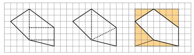
The first two diagrams show the polygon decomposed into triangles and rectangles; the sum of their areas is the area of the polygon. The last diagram shows the polygon enclosed with a rectangle; subtracting the areas of the triangles from the area of the rectangle gives us the area of the polygon.
