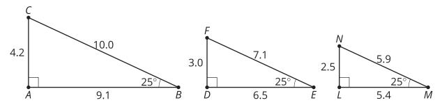
These triangles are all similar by the Angle-Angle Triangle Similarity Theorem. Focusing on the 25 degree angles, we see that all 3 triangles have adjacent leg to hypotenuse ratios of approximately 0.91.
