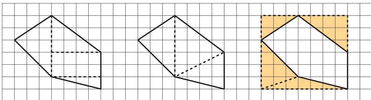
The first two diagrams show the polygon decomposed into triangles and rectangles. The sum of their areas is the area of the polygon. The last diagram shows the polygon enclosed with a rectangle. Subtracting the areas of the triangles from the area of the rectangle gives us the area of the polygon.
