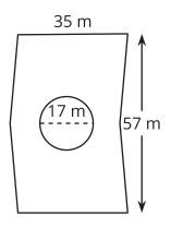
Each floor is the same chevron shape that is approximately 2 parallelograms put together, with the dimensions shown in the image. The circle in the floor plan shows the cross section of the core, which is used to circulate air and carry pipes and wiring throughout the building.
